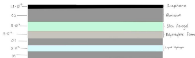
Figure 20 2D Arrangement of shielding layers
